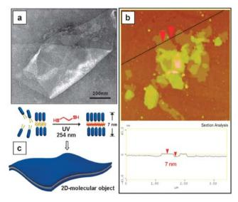
**Fig. 1** (a) TEM image of self-assembled sheets of **1**. (b) AFM image of self-assembled sheets of **1** with height information. (c) Schematic representation of the confined polymerization of 2D peptide sheets.
